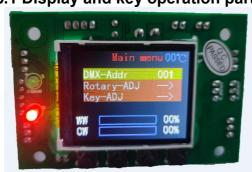
Operational instructions: Under the main menu, press the up and down keys to select different function menus, select different function menus, then press the
